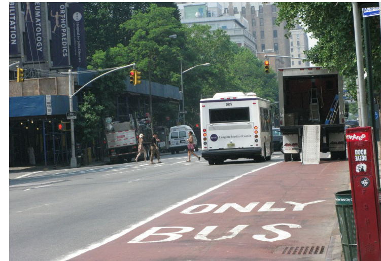
Figure 3.2 -Curbside bus lanes suffer from encroachments by parked cars and delivery vehicles.
