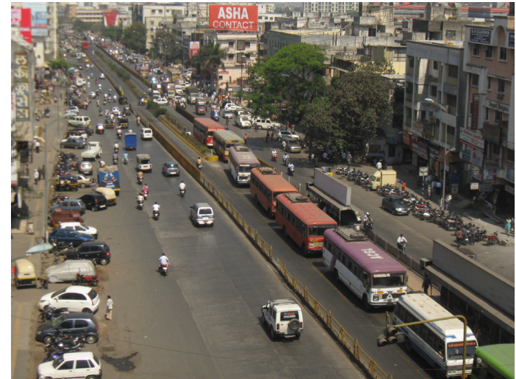
Figure 3.37 -Allowing multiple types of buses to ply in a BRT lane results in slower commercial speeds.
