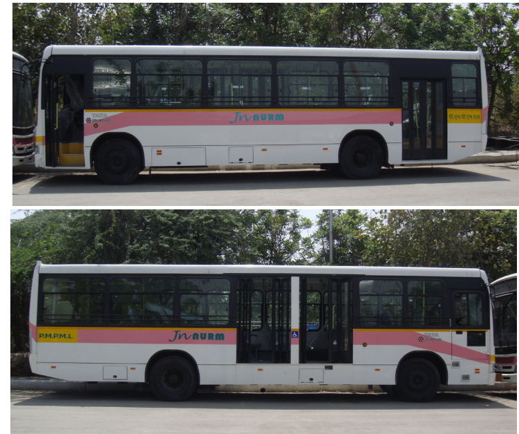
Figure 3.9 -New buses acquired for the Pune Metropolitan Region's BRT system feature modern styling and right-side doors at 900 mm.
