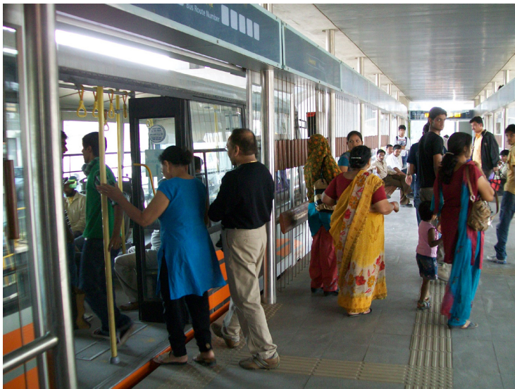
Figure 3.5 -Level boarding on Ahmedabad’s Janmarg system.
