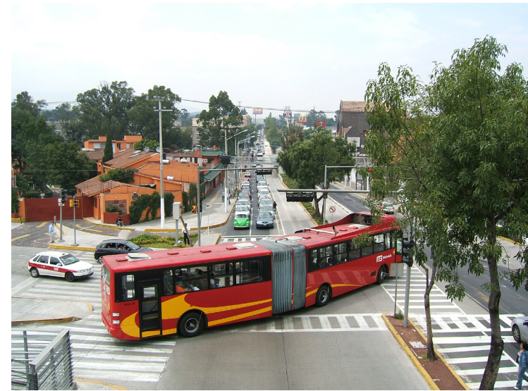
Figure 3.13 - Articulated buses add capacity and reduce congestion in bus lane
