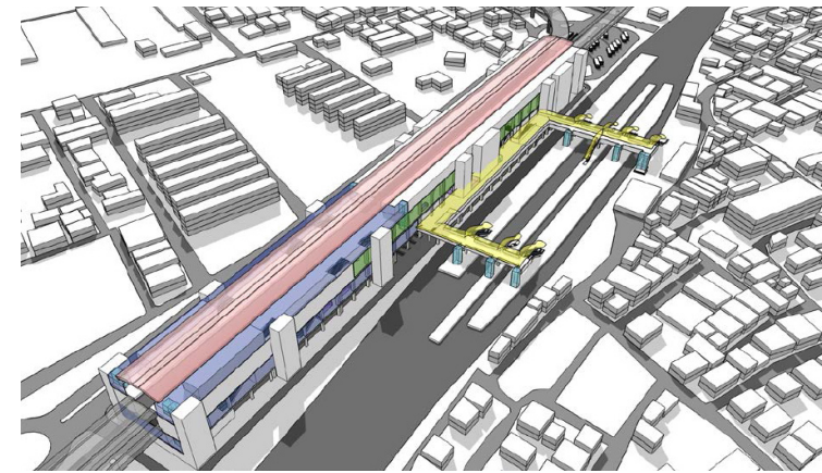
Figure 4.4 -Drawing/visualization showing intermodal integration of St. Thomas Mount Metro Station by Oren Thatcher, Consultant to ITDP
