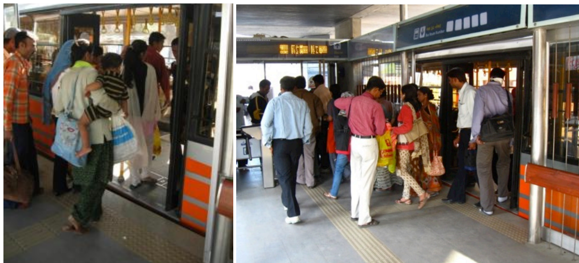
Figure 49: The design of the stations and buses must be coordinated to ensure that floor heights match.
