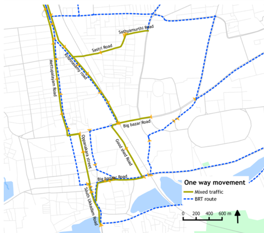
Figure 73: One way movement in Coimbatore CBD for BRT (blue) and mixed traffic (green).
