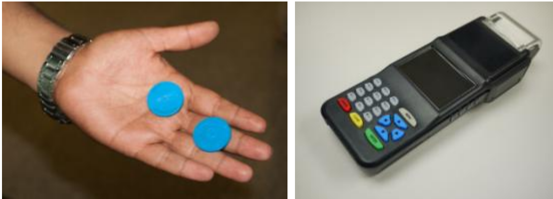
Figure 42: Smart tokens from the Delhi Metro (left), and hand held media reader / encoder with printer (right)
