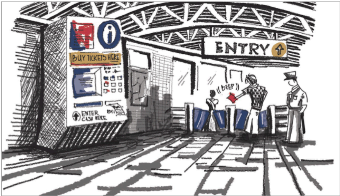
Off-board fare collection. Off-board fare collection reduces travel time, improves the customer experiences, and prevents revenue leakage. A barrier-controlled system with turnstiles allows access when a user taps his/her smart card.
