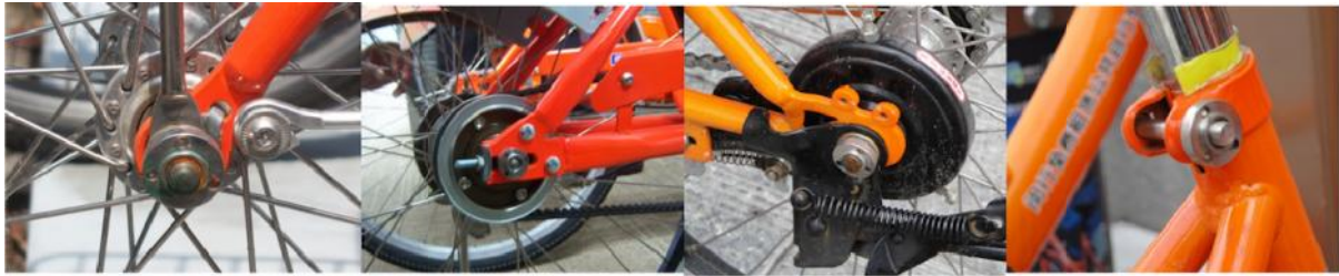
Figure 4. Special parts help deter theft and vandalism.
