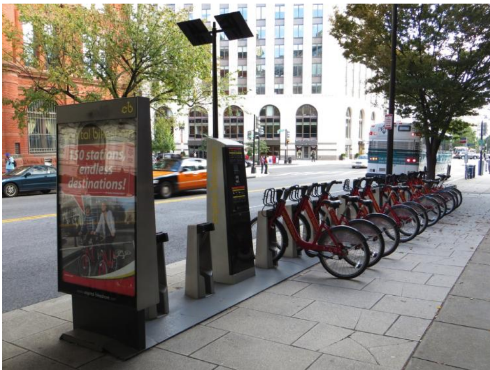
Figure 5. A typical cycle sharing station includes docking positions, a user terminal, and space for advertising.
