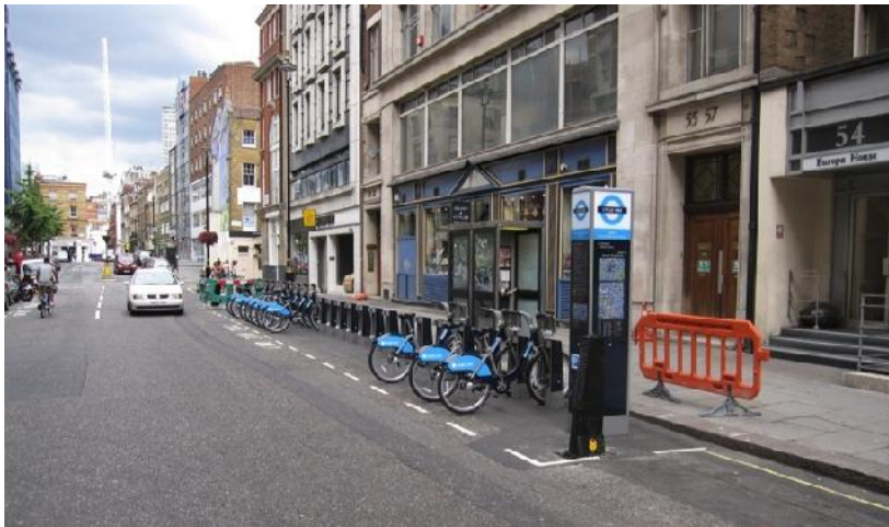
Figure 7. A cycle sharing station can fit in a 2 m wide parking lane.
