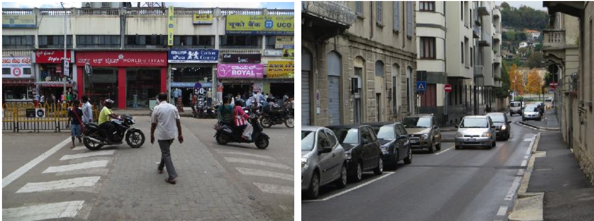
Figure 15. Traffic calming measures such as speed tables (left) and staggered driving lanes (right) can ensure safety for cyclists on streets that are too narrow to accommodate separate cycle tracks.
