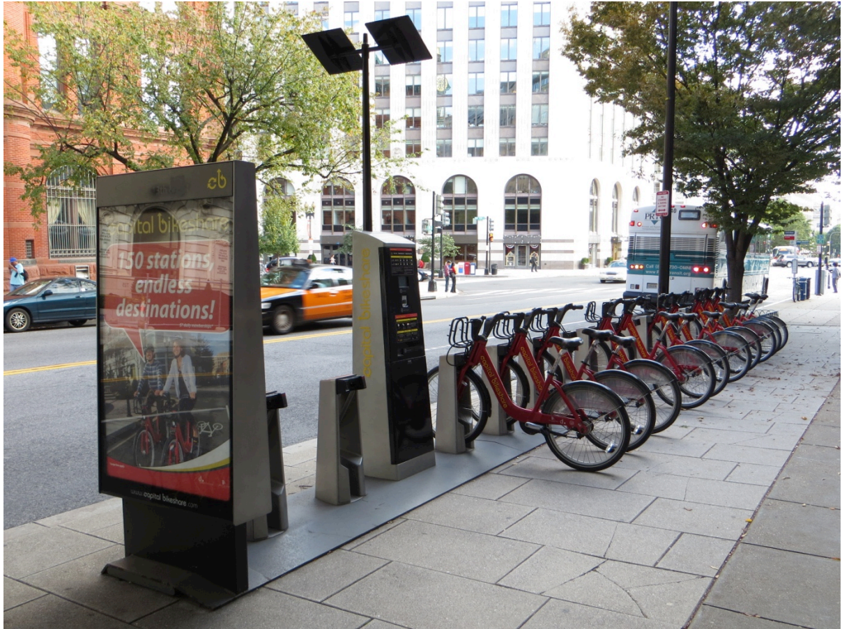
Figure 6. A typical cycle sharing station includes docking positions, a user terminal, and space for advertising.
