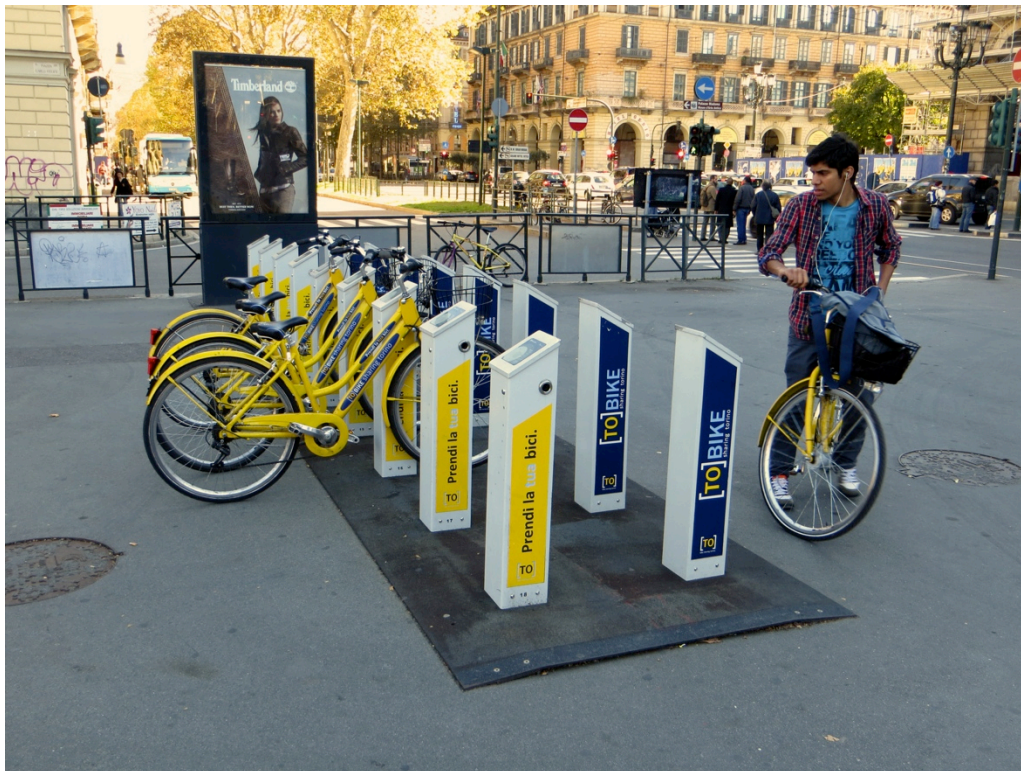
Figure 2. Modern cycle sharing systems feature a dense network of stations. A user checks out a cycle using an RFID-enabled smart card and can return it to any other station.
