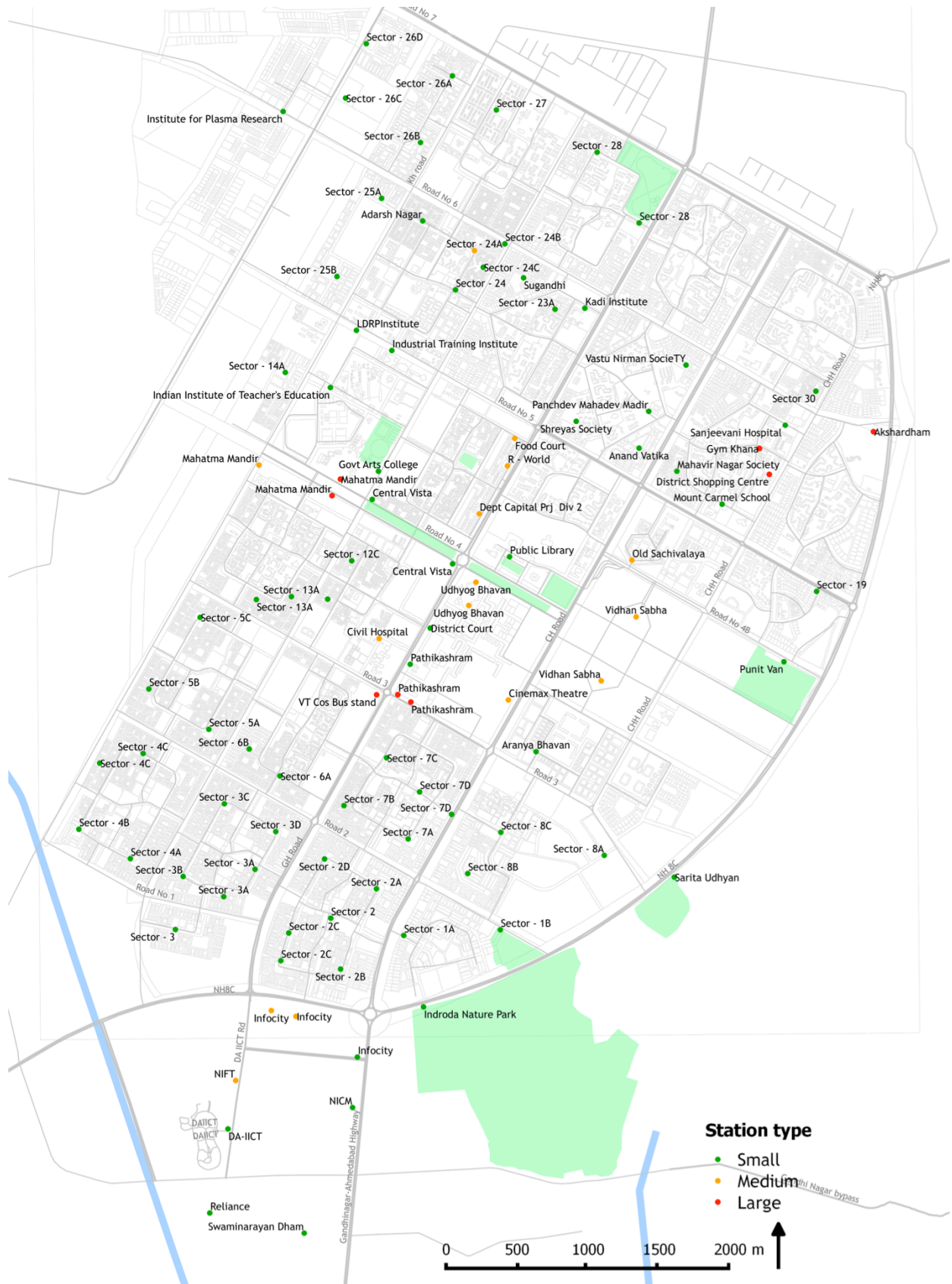
Figure 15. Phase 1 station locations of Gandhinagar cycle sharing system (small = 15 docks, medium = 30 docks, large = 60 docks).
