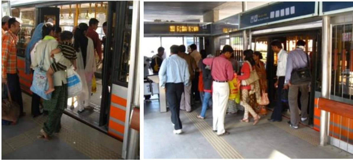
Figure 45: The design of stations and buses must be coordinated to provide level boarding.
