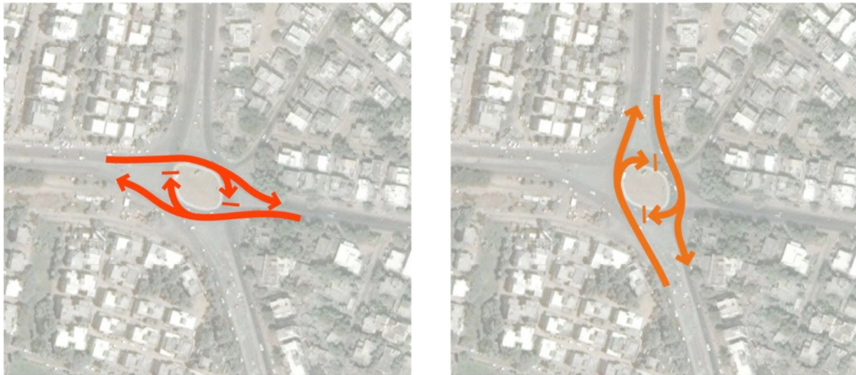
Figure 59: The signal phasing plan for a squareabout. Right-turning vehicles enter the queuing spaces during the first phase and exit ahead of straight-moving traffic during the next phase.
