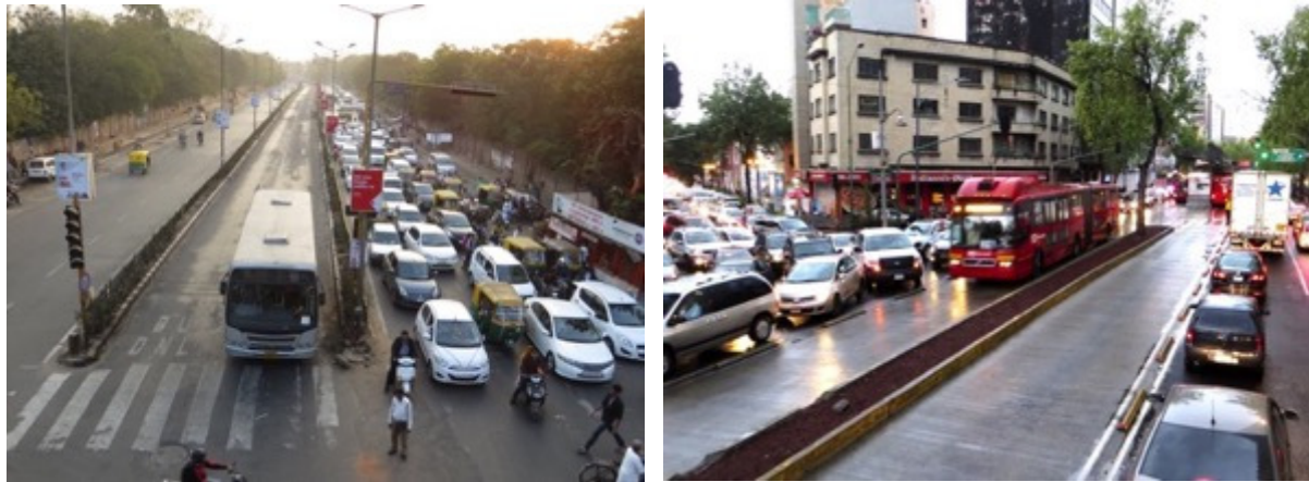
Figure 77: Examples of segregated bus lanes in Ahmedabad (left) and Mexico City (right).
