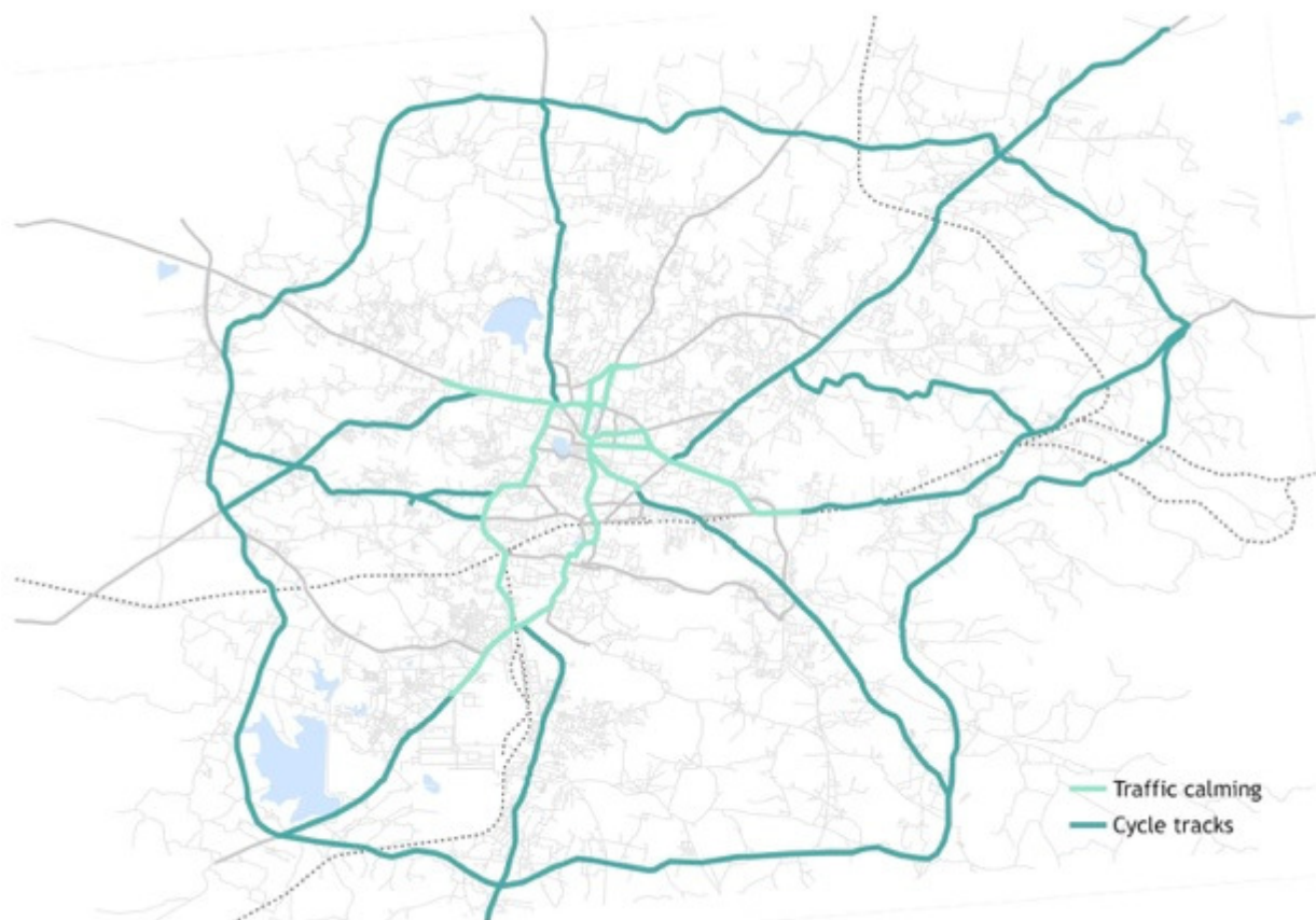
Figure 24: Proposed network of cycle tracks. Where road space is insufficient for separate cycle tracks, traffic calming measures will help ensure that carriageways are safe for cycling.
