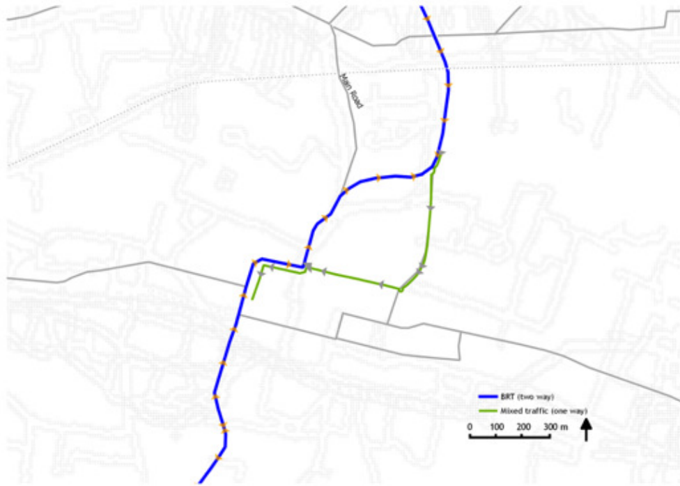
Figure 98: Two-way BRT lanes and one-way northbound mixed traffic from AG More to Rajendra Chowk. The southbound mixed traffic will be made one-way from Rajendra Chowk to AG More via Doranda High Court
