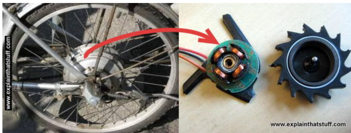
Figure 9: The hub motor of an electric bike
