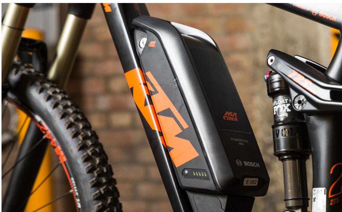
Figure 8: Batteries are generally placed at the down tube
